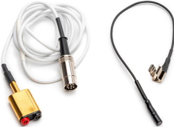
Fig. 5—(Left) CardioPhys™ ECG probe with head stage
