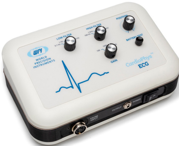
Fig. 1—The CardioPhys™ ECG unit is a bioamplifier
